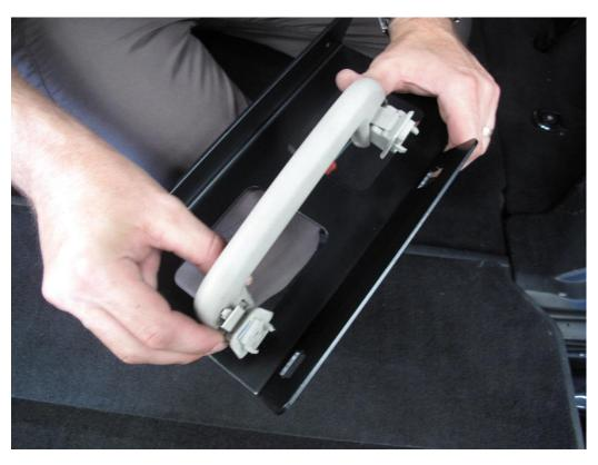
Refit to the vehicle with the supplied self-tapping screws. Ensure the screw enters the clip nut correctly when fitting, if it is not correct the screw will "click" when trying to tighten (Do NOT overtighten)
