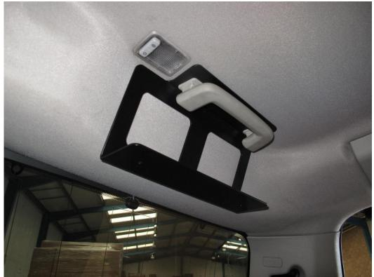
Bracket fitted – NOTE correct orientation for Left and Right hand (R/H shown)
