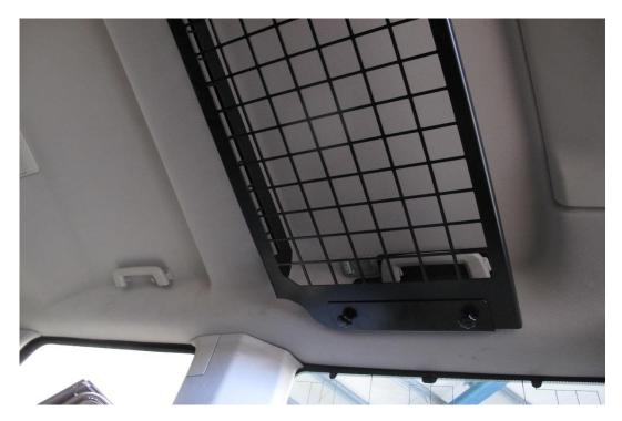
Tighten the thumbwheels by hand ONLY to secure the shelf, ensuring the mounting brackets are flat against the shelf under side.
